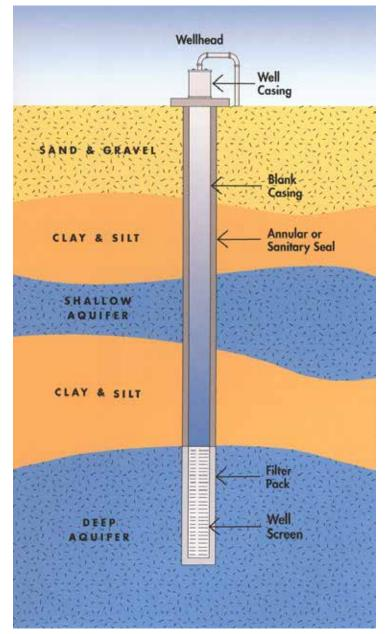
Where the hole intersects the best water producing layers, the driller installs the well casing with thick cuts or perforations. This portion of the well is called the well screen. The well screen allows water to pass into the casing but keeps out sand and gravel. Where the hole intersects layers of clay or fine silt (layers that don't typically produce significant quantities of water), the driller installs un-perforated pipe called blank casing.
